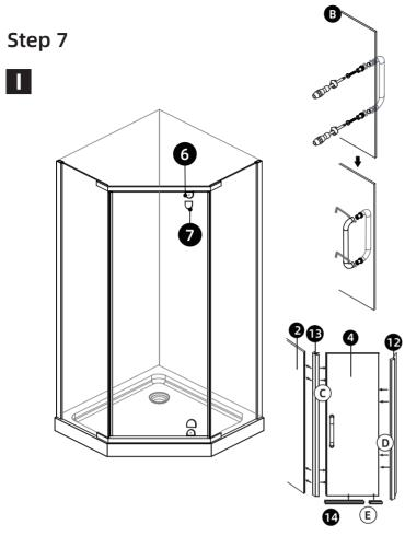
Slide hinge caps (7) over both hinges (6). Hint: Place a small amount of silicone under each cap before installing to ensure cap remain in position permanently This can be done last when sealing the outside of the shower
