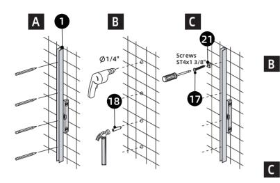
Remove wall jambs and drill 6mm holes with drill bit. Insert plastic wall plugs (18) that are provided. Note: Please use the right fixing for the surface you are screwing into, to ensure the jamb is securely fixed to the wall.
