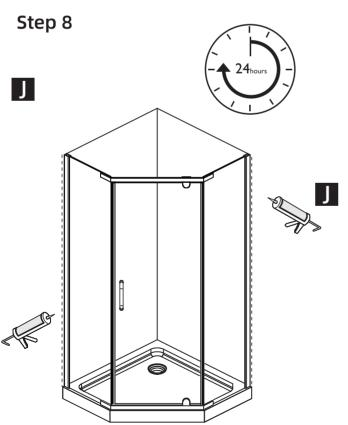
Apply silicone sealer around all external joints of shower screen and allow 24 hours for silicone to set.
